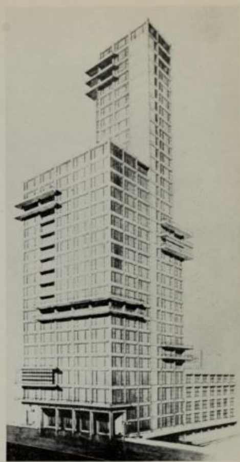
107. Gropius and Meyer. Skyscraper project for the Chicago Tribune tower competition, 1922: an important transitional building in the evolution of Berlin architecture away from Expressionism, it was also the only Tribune competition entry that picked up the structural module of the existing printing works at the back of the offices.
