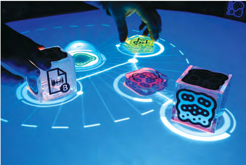
Plate 20 The reactTable is played by manipulating several tangible synthesizer modules on its round interactive table surface. Photo and artwork © Xavier Sivecas.
