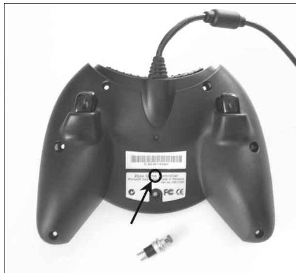
Figure 3.18 Preferred Location for the Reset Button
