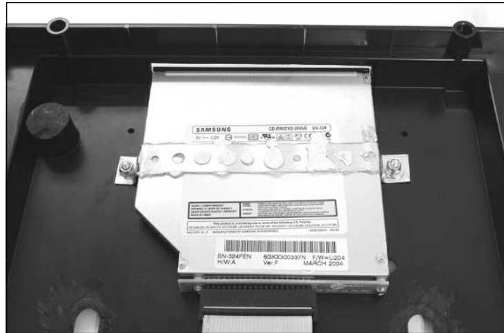
Figure 2.68 The CD-ROM Drive Securely Mounted to the Atari 2600 Bottom Housing
