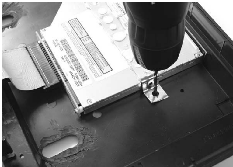
Figure 2.67 Drilling Mounting Holes for the CD-ROM Drive
