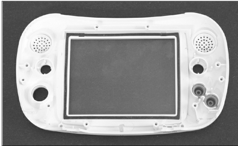
Figure 6.33 GP32 Top Housing with Old Button Membranes Removed
