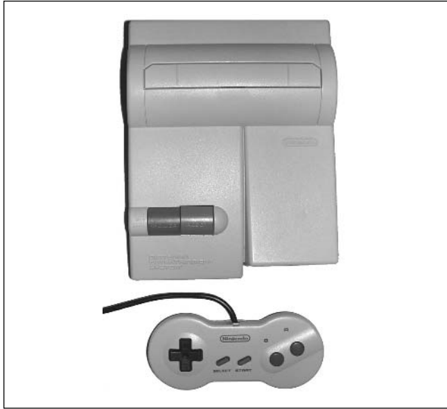
Figure 7.3 The Updated Release of the Nintendo Entertainment System, Also Known as the NES 2 or Top Loader
