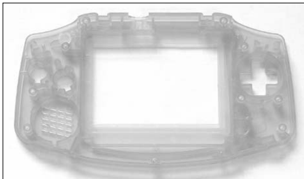
Figure 5.31 Original GBA Housing Ready for Modification
