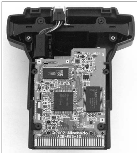
Figure 5.69 Inside the Nintendo e-Reader, Front of Circuit Board
