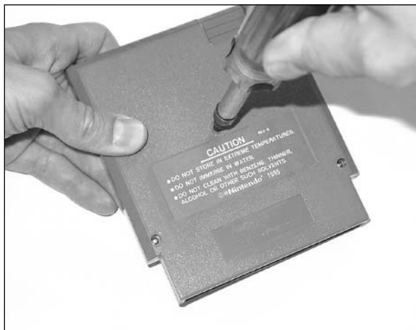
Figure 7.36 Remove the Screws from the NES Game Cartridge
