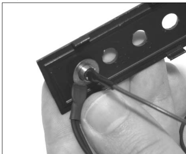
Figure 9.79 Inserting the Ground Connection onto the RCA Connector
