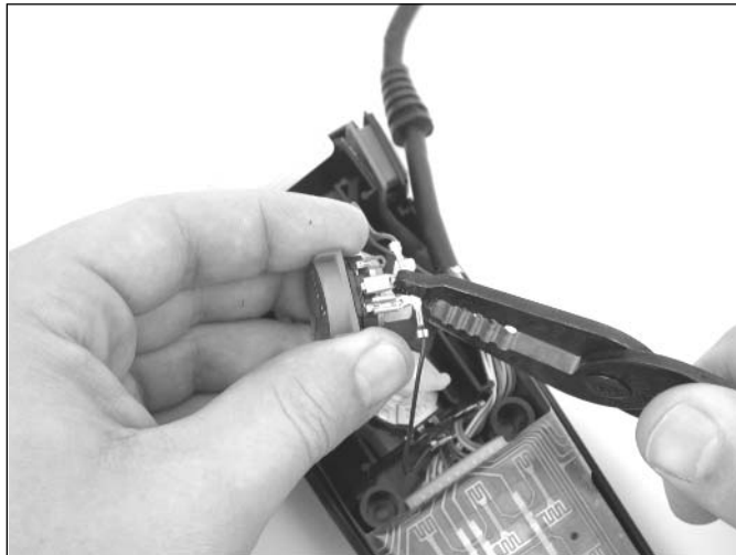
Figure 9.39 Removing Wires from the Upper 5200 Potentiometer
