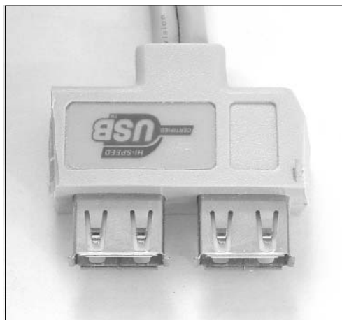
Figure 2.31 Modified USB Backplane
