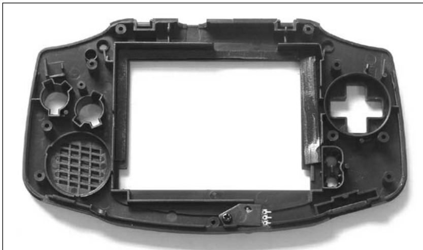
Figure 5.37 Replace the Top Piece of Adhesive Cushion into the GBA
