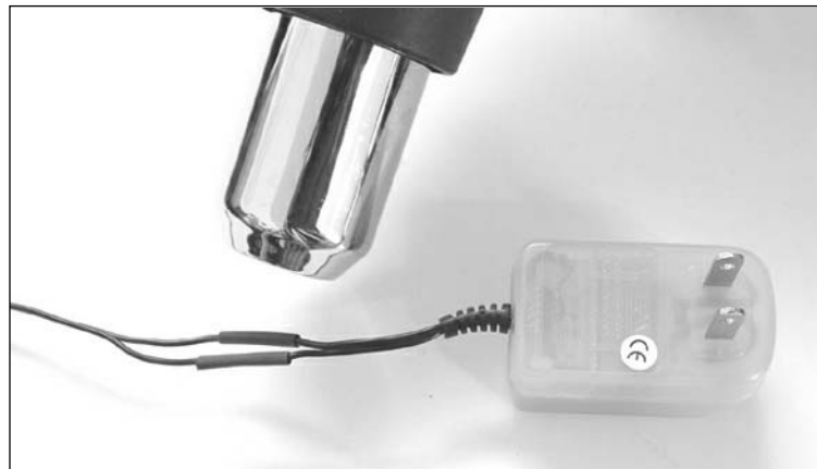
Figure 6.45 Applying Heat to the Heat-Shrink Tubing
