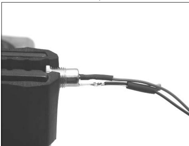
Figure 9.57 Solder the Black Wire and Capacitor to the Connector's Outer Post
