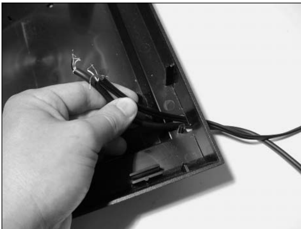
Figure 8.58 Feeding the A/V Cables into the Case
