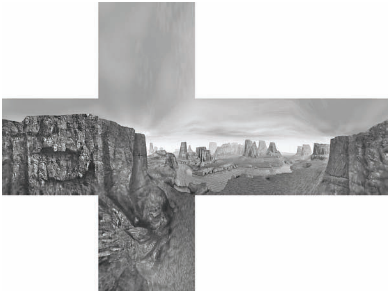
Figure 2.1. A computer-generated New Mexican vista (top) is the result of a series of six seamless textures (bottom) that wrap the skybox to produce the background of Half-Life .
