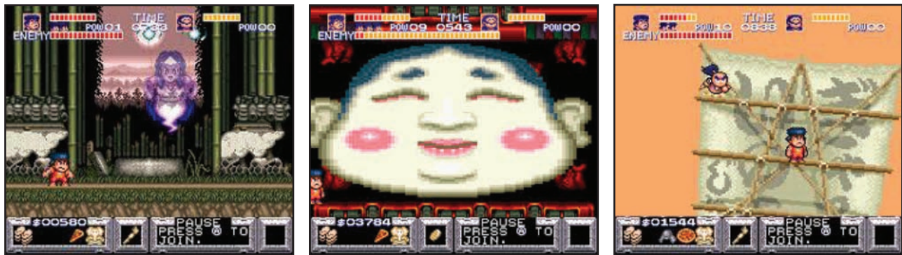
FIGURE 6.21 Screenshots from Konami's The Legend of the Mystical Ninja showcasing the Super Nintendo's color layering and Mode 7 scaling and rotation effects.
