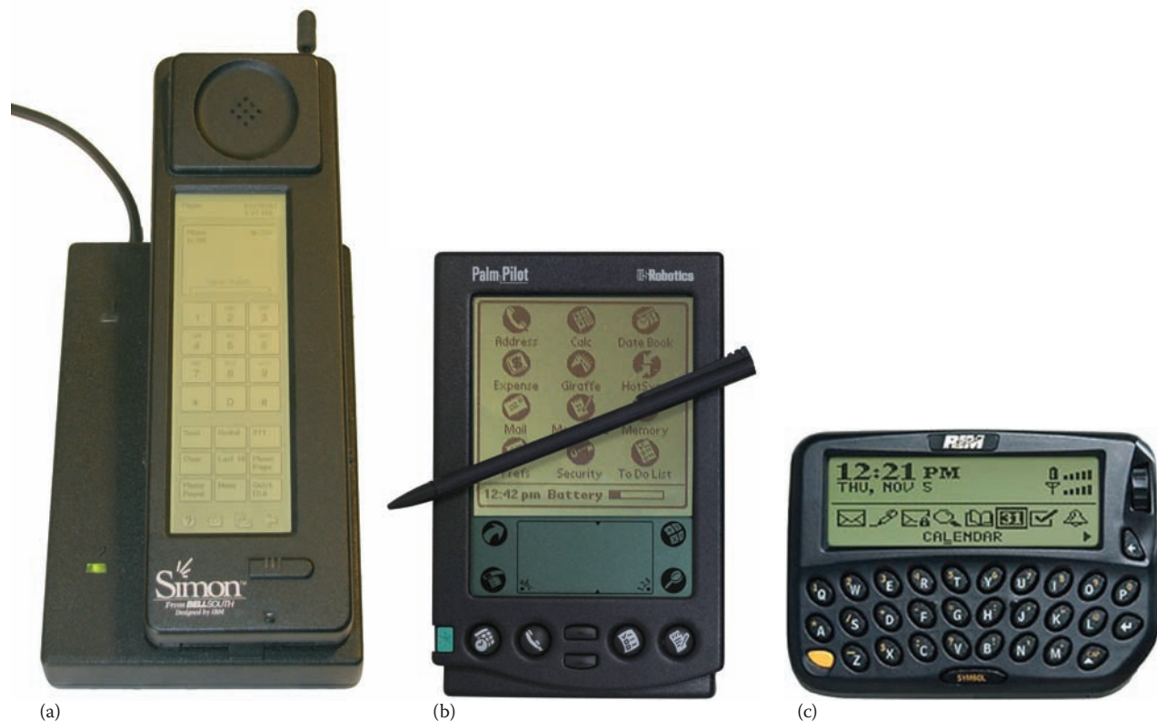
FIGURE 14.1 “Smart” devices: (a) IBM Simon, (b) PalmPilot with stylus, and (c) BlackBerry 850 pager.
