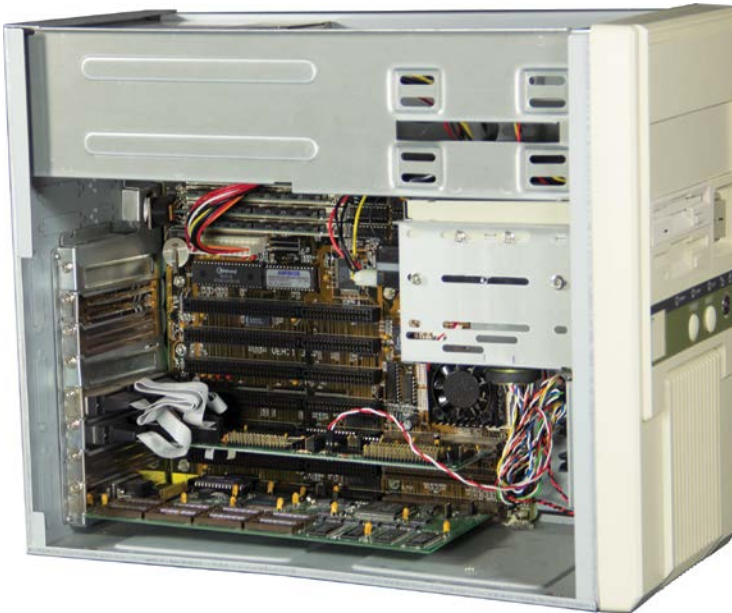
FIGURE 6.12 Interior of an IBM compatible PC from the mid-1990s showing the open architecture concept.
