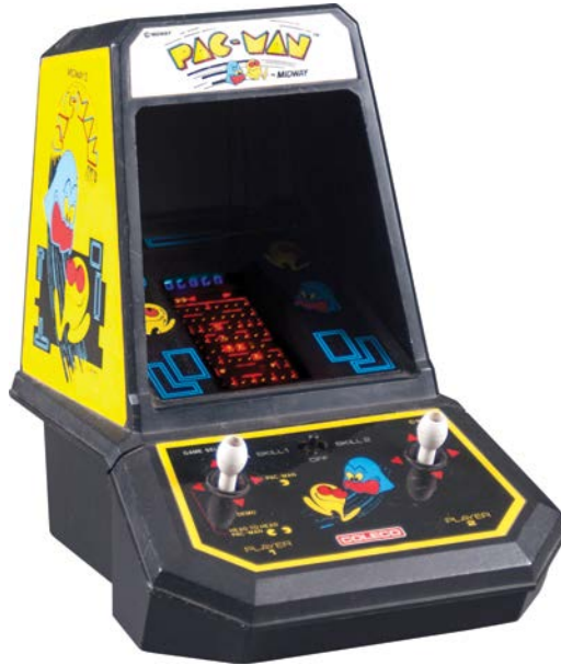
FIGURE 5.4 Coleco's Mini Arcade cabinets used VFD technology to create bright colors that other small LED and LCD units could not replicate.
