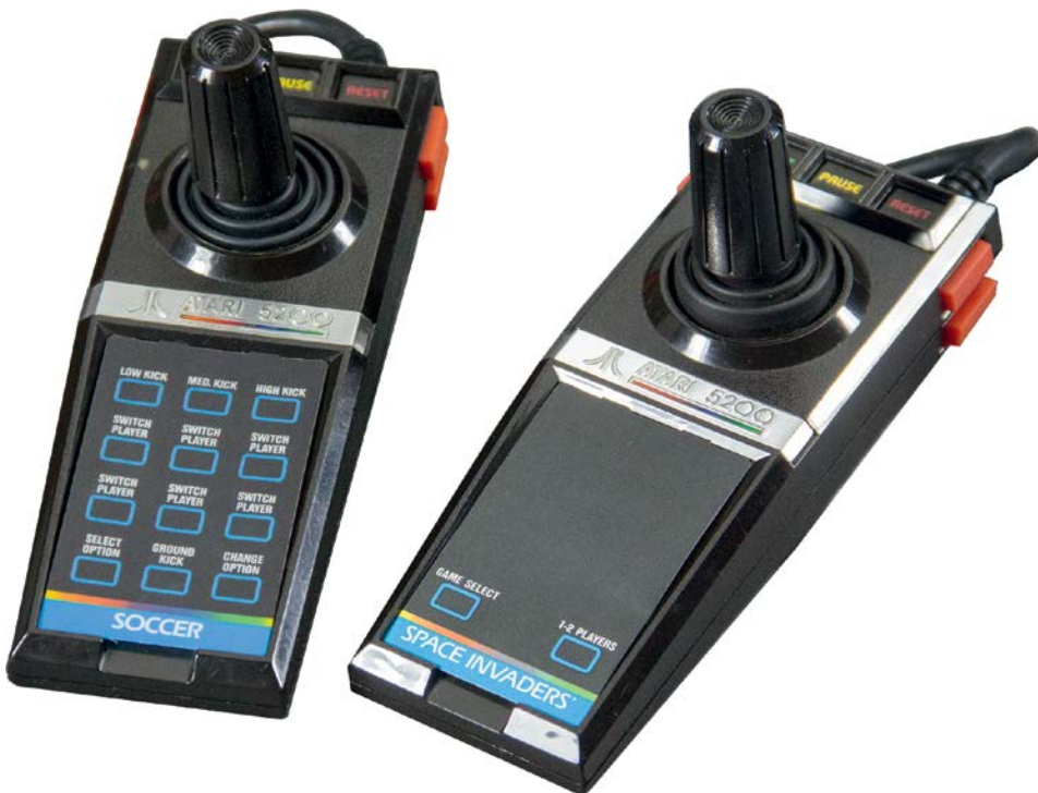
FIGURE 5.7 Atari 5200 Super System Controllers with overlays for Space Invaders and Soccer . Each reveals the different input needs of each game.
