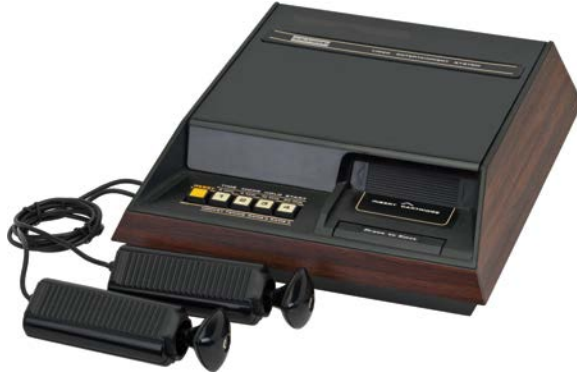
FIGURE 5.1 Fairchild Semiconductor released the first true cartridge-based home console in 1976. The main unit, designed by engineer Jerry Lawson, contained a number of built-in games as well as a cartridge port. The most notable feature of the unit was its unconventional controllers that combined a push button and rotary-like directional controller on a stick. (Photo Evan Amos. CC BY-SA 3.0.)
