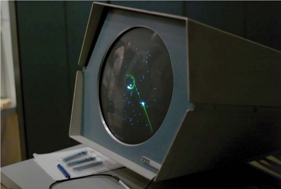
FIGURE 2.3 Spacewar! played on a PDP-1 minicomputer. The trails of green and yellow left by the ships in the image are phosphorescent artifacts of the PDP-1’s CRT scope. (Photo by Joi Ito. CC BY 2.0. Level adjustment from original.)
