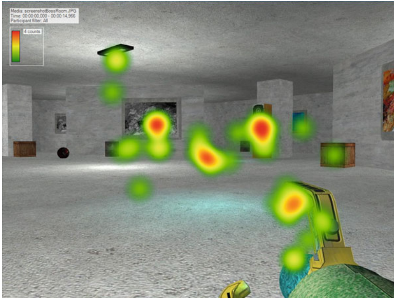
Fig. 25.1 Example heatmap from one participant viewing game stimuli for 15 s. The visual representation of clustered areas indicate locations of a higher number of fixations
