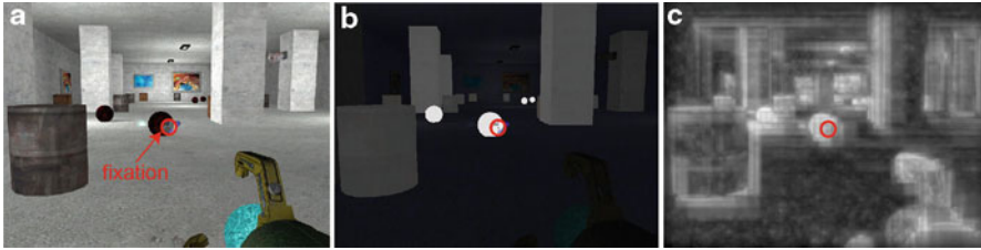
Fig. 25.9 Predicting visual attention from fixation statistics: (a) An example reconstructed framebuffer of the game is overlaid with the visualization of a fixation in the current frame. In Figure (b), fixation statistics were used to predict the importance for each object in the scene which is visualized by the brightness of the objects (brighter objects are more important than darker ones). Figure (c) shows the corresponding saliency map. Since fixation statistics account for semantics, they can predict better the high importance of doors or objects in the center, while saliency maps are less selective and predict the importance of pixels rather than objects
